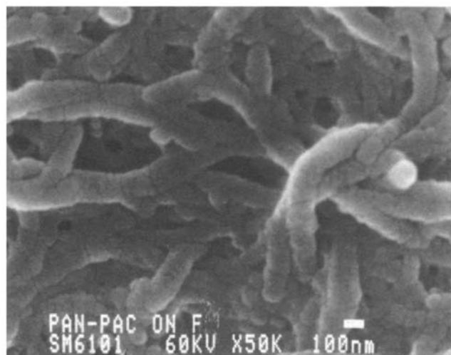
Fig. 1 SEM of long fibrils captured by membrane filter. These fibrils contain polyaniline–poly(acrylic acid) complexes.
